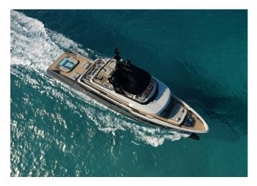
Two Caterpillar C 32 of 970 kW each will allow it to run at a maximum speed of over 14.5 knots. Fuelled by tanks of 60m³ approximate capacity, at economic speed this boat will reach a 4,000 mile range. Two watermakers producing about 8.6m³/day will feed the 10m³ total capacity of the freshwater tanks. The yacht is equipped with two pairs of stabilizers ensuring optimal performance both at anchor and underway.
