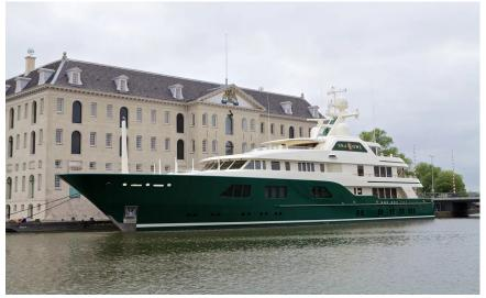
She also has accommodation for 18 crew members, including the ship's captain. Sea Owl has a steel hull and an aluminium superstructure. She is powered by 2 MTU engines, which give her a top speed of 16 kn. The yacht carries 147,726 litres of fuel on board.
