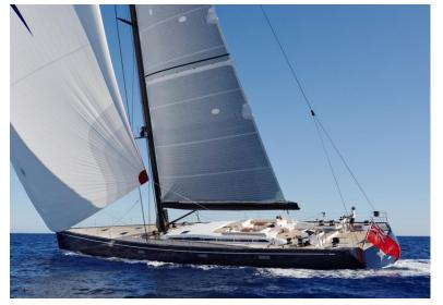
A twin helm is an ideal configuration for racing while below the waterline lies a hydraulic lifting keel that works threefold to maximise comfort, enhance performance and allow owners to access shallower anchorages and ports. Fully extended, she has a draft of 5.75 metres that retracts to 3.55 metres.
