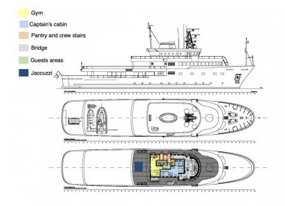
Tribu comfortably cruises at 12 knots, reaches a maximum speed of 15 knots with a range of over 6,000 nautical miles from her 101,000 litre fuel tanks. Her water tanks store around 20,000 Litres of fresh water. She was built to RINA ( Registro Italiano Navale) C & HULL • MACH classification society rules.
